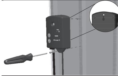
Mount using the keyhole on the back of the unit.
