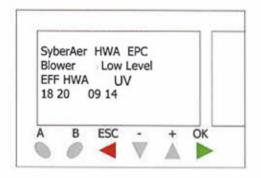
The alarms will be displayed on the screen in the position they are displayed above. The first line will show the SyberAer HWA and EPC, the second line will show the SyberAer Blower and Low Level. The third line will show the Effluent Tank HWA and the UV.
