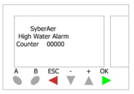
This Screen will show you the number of High Water Alarms that have occurred in the SyberAer tank. This value can be reset by pressing the – button for 3 seconds.
