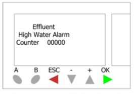
This Screen will show you the number of High Water alarms that have occurred in the Effluent tank. This value can be reset by pressing the – button for 3 seconds.
