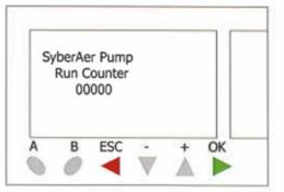
This Screen will show you the number of times the SyberAer Pump has been turned on by the logic. The Pump Test Switch will not count. This value can be reset by pressing the – button for 3 seconds.
