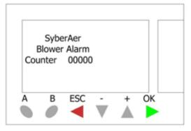
This Screen will show you the number of Blower alarms that have occurred in the SyberAer tank. This value can be reset by pressing the – button for 3 seconds.
