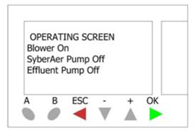
This screen will show the status of the motors in the system. Blower On/Off SyberAer Pump On/Off Effluent Pump On/Off
