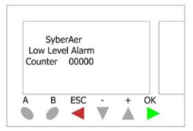
This Screen will show you the number of Low Level alarms that have occurred in the SyberAer tank. This value can be reset by pressing the – button for 3 seconds.
