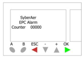
This Screen will show you the number of EPC alarms that have occurred in the SyberAer tank. This value can be reset by pressing the – button for 3 seconds.
