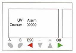
This Screen will show you the number of UV alarms that have occurred This value can be reset by pressing the – button for 3 seconds.
