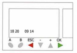
The information shown in the bottom of the screen when an alarm comes on is the time and Date.  $18\ 20 = 6:20$ PM and  $09\ 14 =$  Sept 09. This is at the time the alarm starts. If there are multiple alarms (HWA and EPC in the SyberAer) the date and time captured will be when the first alarm came on.
