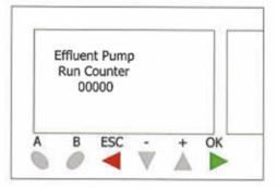
This Screen will show you the number of times the Effluent Pump has been turned on by the logic. The Pump Test Switch will not count. This value can be reset by pressing the – button for 3 seconds.
