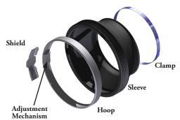
**Sleeve:** The sleeve is designed for flexibility in all dimensions to accept some movement between the pipe and the structure. Sleeves are manufactured with EPDM which provides for protection against ultraviolet degradation while the structure is awaiting installation. The sleeve is available in Nitrile for use in applications requiring oil-resistance. Sleeves are designed for use with either single or dual take-up clamps.
