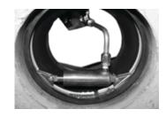
Using the hand pump, extend the jack cylinder until the tongue engages the first slot while holding the connector secure with one hand. At this point the connector need no longer be manually secured.
