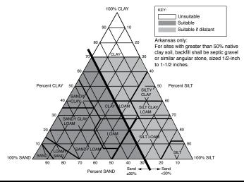
b) For a tank soil cover depth that is greater than 2.0 feet and up to 4.0 feet (600 to 1,200 mm), suitable soil textures include:
